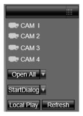
Figure 3-4 Monitor Channel Menu Tree
